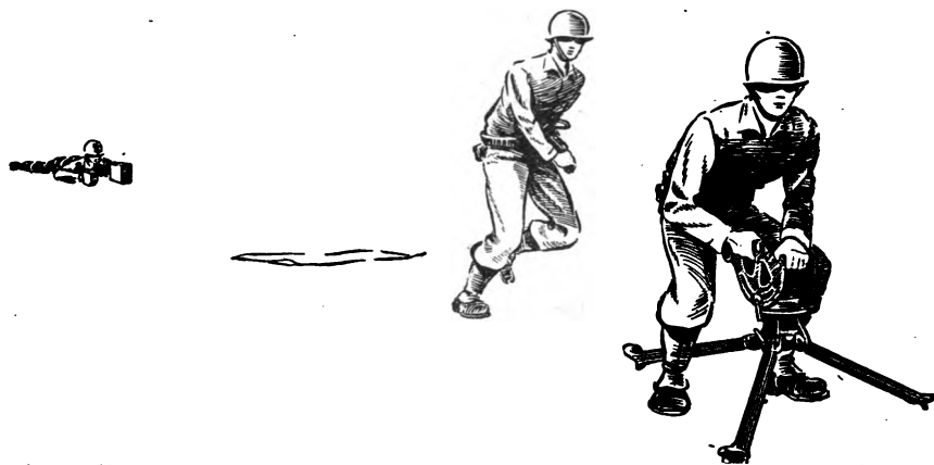
Figure 52. No. 1 removes his right hand from the trail leg. Still grasping the gun pintle housing with his left hand, he places his left forearm over his left thigh to steady the tripod, and glances up to see that the trail leg is aligned in the direction of fire. No. 2 starts forward.
