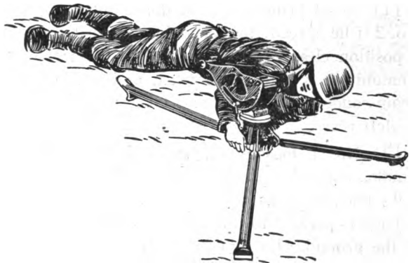
Figure 71. No. 1 supports the pintle socket in the palm of his left hand, sees that the trail leg is in the direction of fire, levels the dial, and with his right hand clamps both front legs, the right leg being clamped first. No. 2 crawls forward, cradling the gun in the bend of his elbows.
