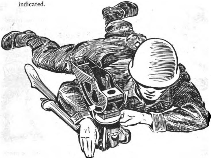
Figure 69. No. 1 uses both hands to loosen the front leg jamming handles.
